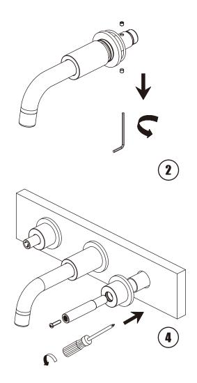
Once the front wall is finished, remove the protective caps for installing the trim.
